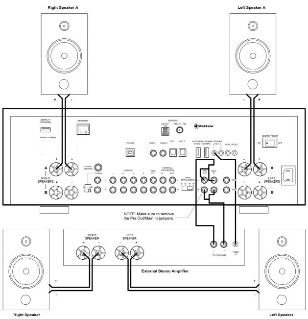
Option 2: Using an External Amplifier and the RR 2180's Internal Amplifier
